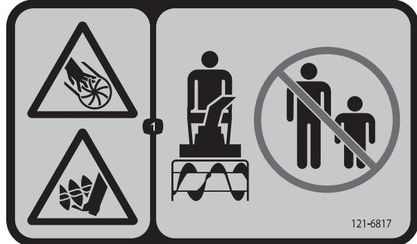
1. Cutting dismemberment, impeller and cutting dismemberment, auger hazards—keep bystanders a safe distance from the snowblower.
