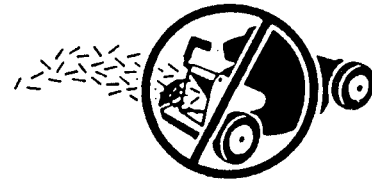
Never open chute door on mower when engine is running, unless grass bag or optional side discharge attachment is installed
