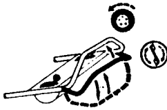
Squeeze control bar against handle to engage blade and traction drive
