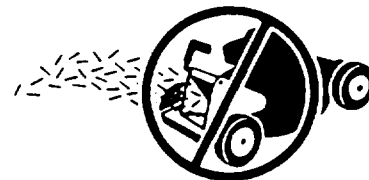
Never open chute on mower when engine is running, unless grass bag or optional side discharge attachment is installed
