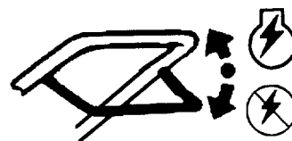
Squeeze control bar against handle to drive
