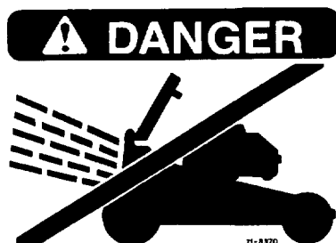
Never open discharge door on mower when engine is running, unless grass bag, optional side discharge attachment or optional mulching plug is installed
