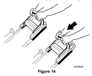
**Note:** If the machine does not freely roll backward after self-propelling, stop walking, hold your hands in place, and allow the machine to roll a couple of inches/centimeters forward to disengage the wheel drive. You can also try reaching just under the personal pace handle to the metal handle and push the machine forward a couple of inches/centimeters. If the machine still does not roll backward easily, contact an Authorized Service Dealer.
