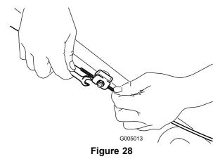
2. Pull down the cable jacket (toward the machine) until there is no slack in the cable (Figure 29).
