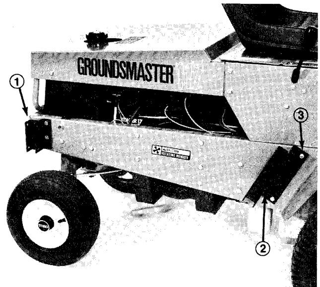
Figure 15 1. Rear bracket 3. Reinforcing plate on this screw (inside frame) 2. Front bracket
