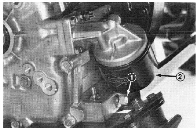
Figure 21 1. Drain plug 2. Oil filter
