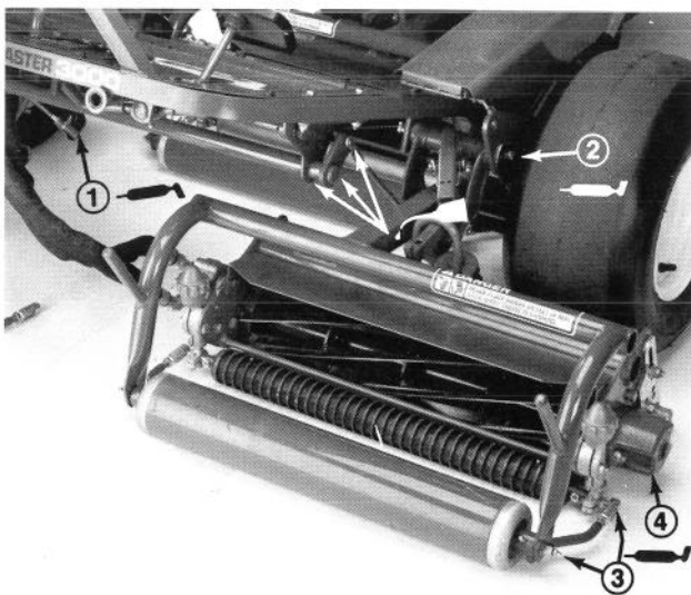
Figure 29 1. Mow pedal pivot 2. Lift arm pivot 3. Pull frame roller 4. Refer to cutting unit manual
