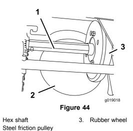
**Important:** Do not get oil on the rubber wheel or the steel friction pulley because the traction drive will slip (Figure 44).
