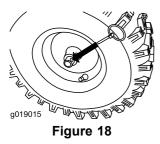
To self-propel, axle pin through the holes in the wheel hubs and the inner axle holes (Figure 19).
