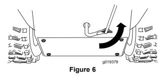
6. Pull up on the speed control rod and insert the trunnion into the hole in the speed selector lever (Figure 5).
