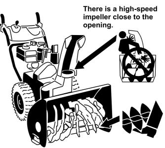
The low-speed auger has a moving pinch point close to the opening.
