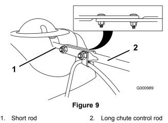
4. Insert the front end of the rod into the opening in the back of the chute gear cover until it slides into the chute gear (Figure 10).
