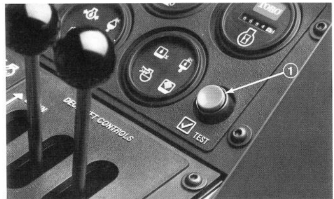
Figure 12 1. Warning Light Check Switch
