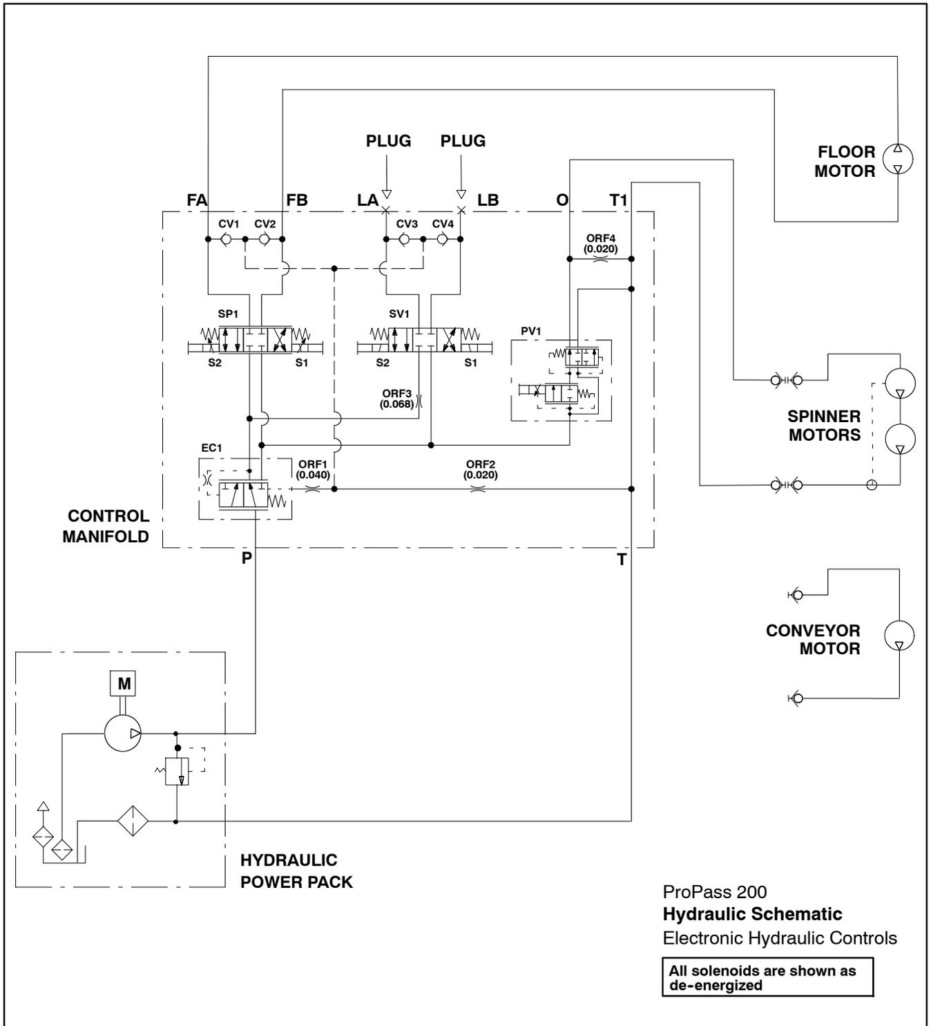
**NOTE:** The hydraulic schematic shown above includes the hydraulic power pack as the hydraulic supply source. If your ProPass uses hydraulic supply from the tow vehicle, the vehicle includes the hydraulic pump, relief valve and hydraulic reservoir that are used for the ProPass.
