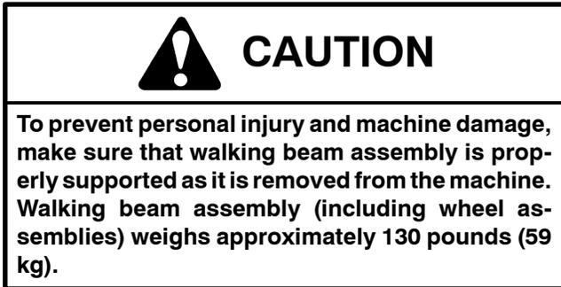
3. Support walking beam assembly to prevent it from shifting during removal.
