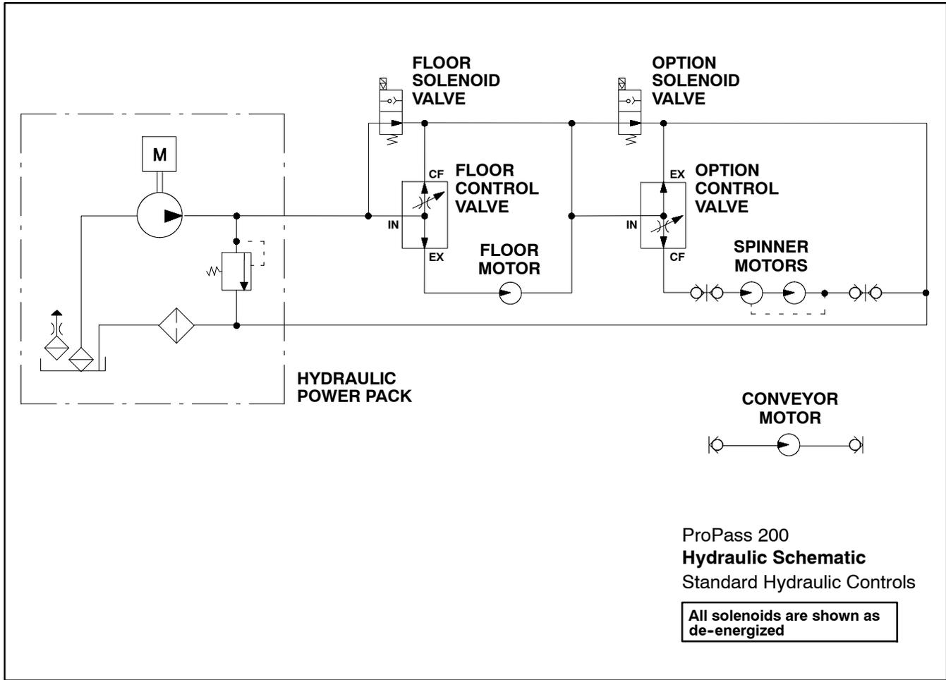
**NOTE:** The hydraulic schematic shown above includes the hydraulic power pack as the hydraulic supply source. If your ProPass uses hydraulic supply from the tow vehicle, the vehicle includes the hydraulic pump, relief valve and hydraulic reservoir that are used for the ProPass.
