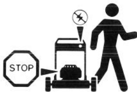
Stop engine before leaving operator position
