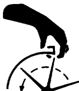
Shut off engine before unclogging discharge chute
