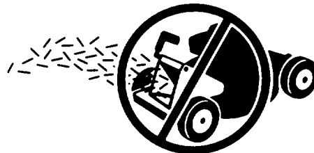
Never open chute door on mower when engine is running, unless grass bag or side discharge attachment is installed
