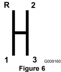
**Important:** Do not shift the transaxle to the reverse or forward gear unless the vehicle is standing still. Damage to the transaxle may occur.
