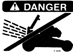
Never open chute door on mower when engine is running, unless grass bag or side discharge attachment is installed
