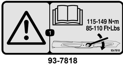
1. Warning—read the *Operator's Manual* for instructions on torquing the blade bolt/nut to 115-149 N-m (85-110 ft-lb).
