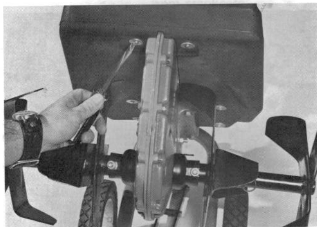
Figure 27 Removal of Screws Holding Shroud
