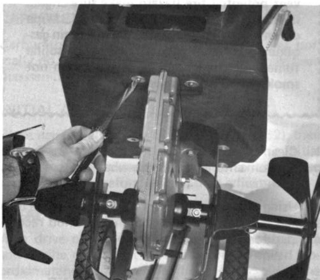
Figure 25 Removal of Screws Holding Shroud
