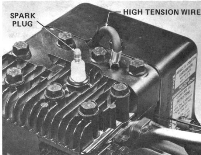
Figure 19 High Tension Wire in V Notch
