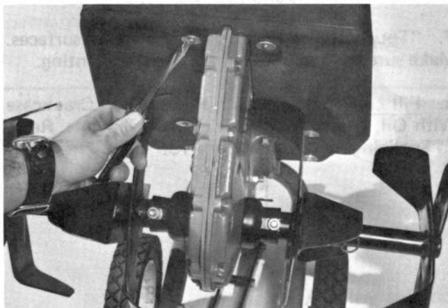
Figure 30 Removal of Screws Holding Shroud
