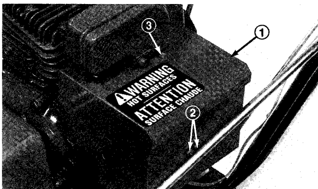
Figure 20 1. Heater box 2. Phillips screws 3. Hex head screw
