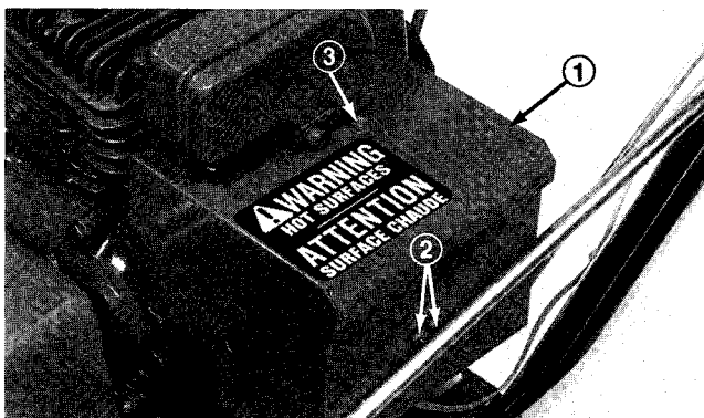
Figure 20 1. Heater box 2. Phillips screws 3. Hex head screw
