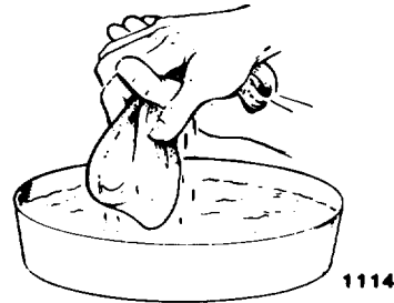
Precleaner service - wash, squeeze dry, coat with oil & wring out
