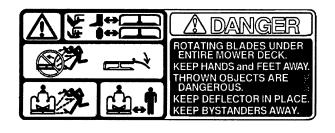
ON THE INNER SHIELD (Part No. 92-7108)
