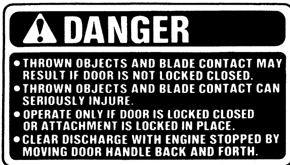
ON DISCHARGE TUNNEL
