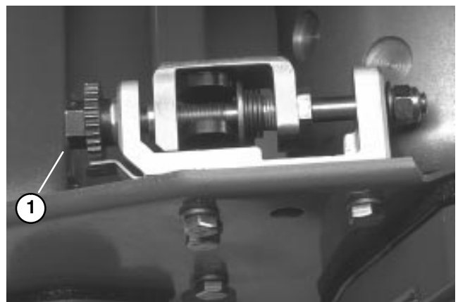
Figure 9 1. Bedbar adjusting screw
