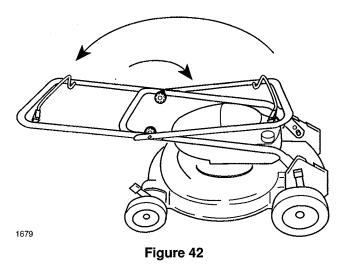
5. Loosen knobs securing top handle section to bottom section and fold top handle section back towards rear of mower into storage position.
