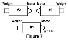
**Note:** Counterweights are shipped installed to the right end of the verticutters. The bolts on the left end are to be used for securing the hydraulic motor.
