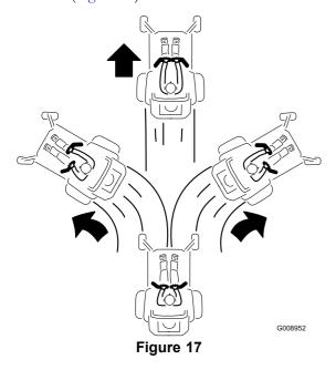
To go straight, apply equal pressure to both motion-control levers (Figure 17).
