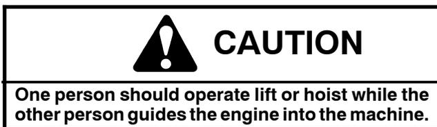
**IMPORTANT: Make sure not to damage the engine, fuel and hydraulic lines, electrical harness, or other parts while installing the engine.**
