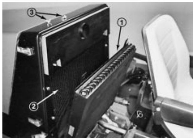
Figure 41 1. Oil Cooler 2. Radiator 3. Wing Nuts
