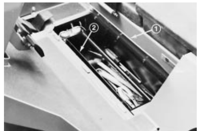
Figure 20 1. Hinged Floor Plate 2. Removable Tool Tray
