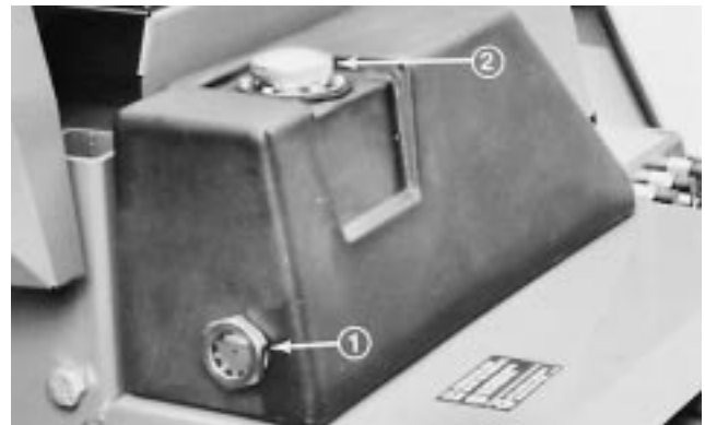
Figure 6 1. Hydraulic Oil Level Sight Glass 2. Reservoir Fill Cap
