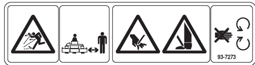
ON CUTTING UNITS, UNDER COVERS (Part No. 93-7273) Replaces Decal Part No. 67-5360 for CE
