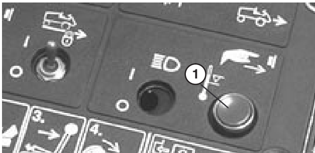
Figure 30 1. Engine Over-ride Button
