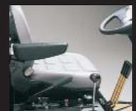
A single foot pedal for forward or reverse, plus standard speed control, make operation easy. Drivers appreciate the two-piece adjustable seat and controls that are easy to see and use.
