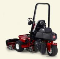
**Perfect tri-cycle design.** The rear wheel is engineered to track within the radius of the front wheels to keep the operator safe on sharp turns near bunkers.
