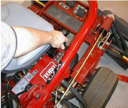
Check the control linkage for improper adjustment, binding or broken parts.
