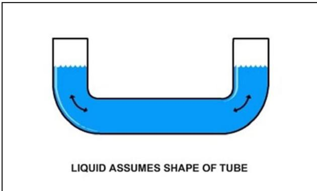
A liquid can assume any shape and be bidirectional. Fluid is able to flow in any and all directions within a container.
