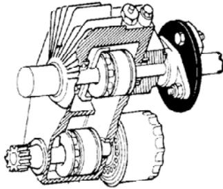
A similar version is the U-type transmission. In this type of system the pump and motor are constructed as a common component with the pump usually located above the motor.
