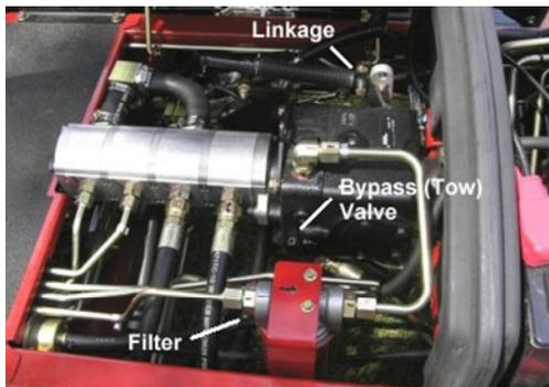
The hydrostatic transmission will provide trouble free operation if it is serviced and maintained properly. There are, however, a few simple items that are often overlooked when poor performance is evident.
