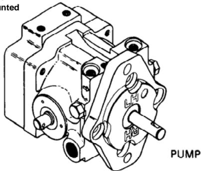
The first type is a hydrostatic system which consists of a hydrostatic pump with a remotely mounted motors. In this type of hydrostatic system the hydrostatic pump is mounted by, and driven by, the units engine. The pump is connected to the drive motor by hoses or steel lines. These motors can be mounted directly to the wheels or to a drive axle.
