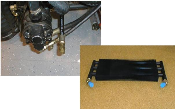
Put caps or plugs on any hydraulic lines left open or exposed during testing or removal of components.
