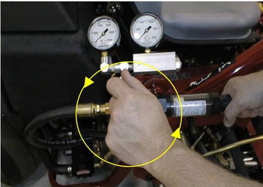
To minimize the possibility of damaging the components, completely open the load valve by turning it counter clockwise (tester with pressure and flow capabilities).
