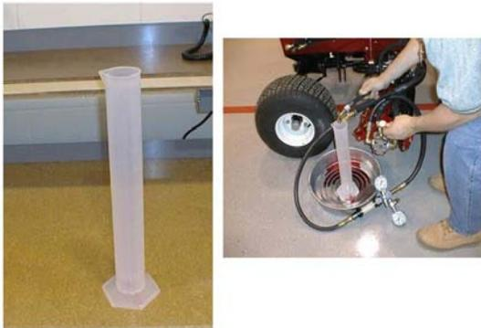
This measuring cylinder is used to measure flow on very low flow circuits. An example is measuring the flow from the case drain line of a hydraulic motor to test for motor efficiency.
