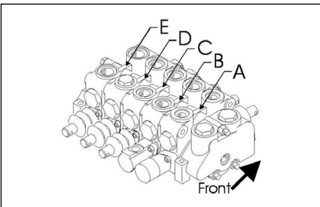
This is that same spool valve, assembled with multiple sections to make a valve bank or assembly. This example is from a Greensmaster riding mower. In this example the valve bank would control all of the hydraulic functions on the machine and would be actuated by foot or hand operated levers.
