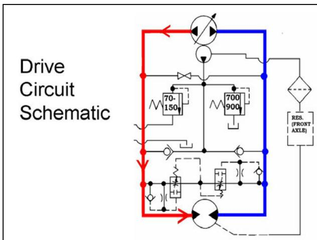
Here is the closed loop circuit of an inline hydrostatic transmission shown in a schematic view.
