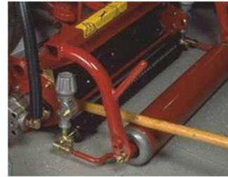
Here we have put a stick into the cutting reel to prevent the reel motor from turning.
