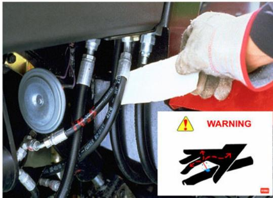
Before disconnecting or performing any work on a hydraulic system, all pressure in the system must be relieved by stopping the engine and lowering or supporting the implement.
