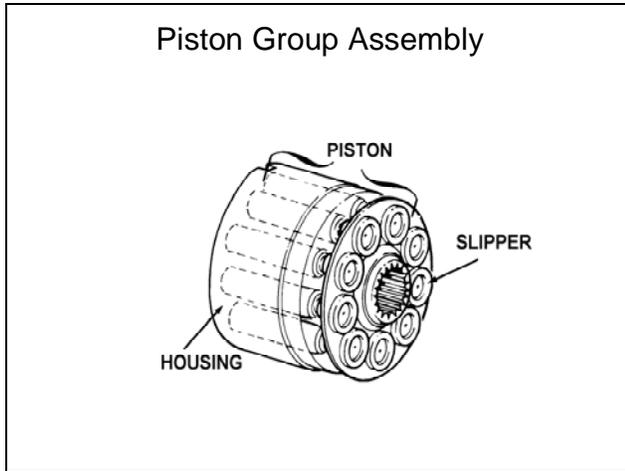
The pump consists of the following components:
