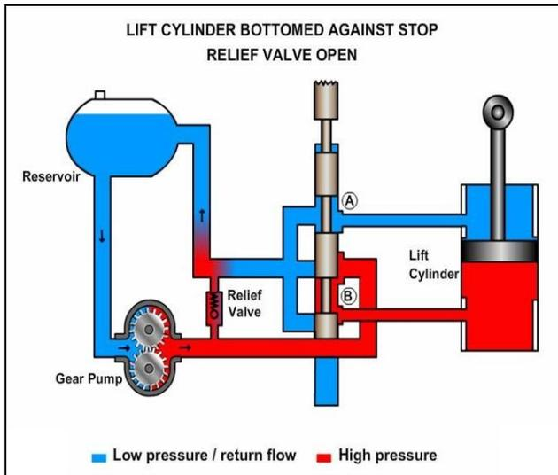
Since the fluid from a positive displacement pump must flow continuously whenever the pump is running, it must have some where to go if not being used by the actuators. If the load on the cylinder becomes too great or if the ram bottoms out, the flow from the pump will be directed past the relief valve returning to the reservoir.
