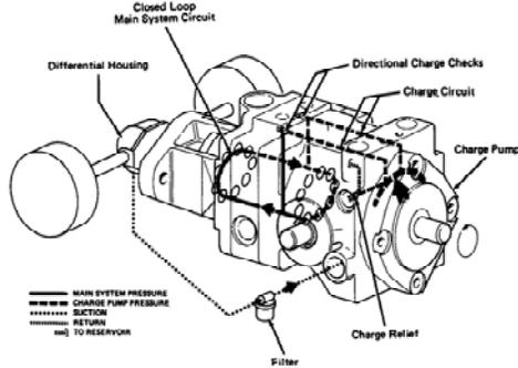
Here is a view of the closed loop main circuit and charge circuit within the inline hydrostatic transmission from a Groundsmaster 300 Series.
