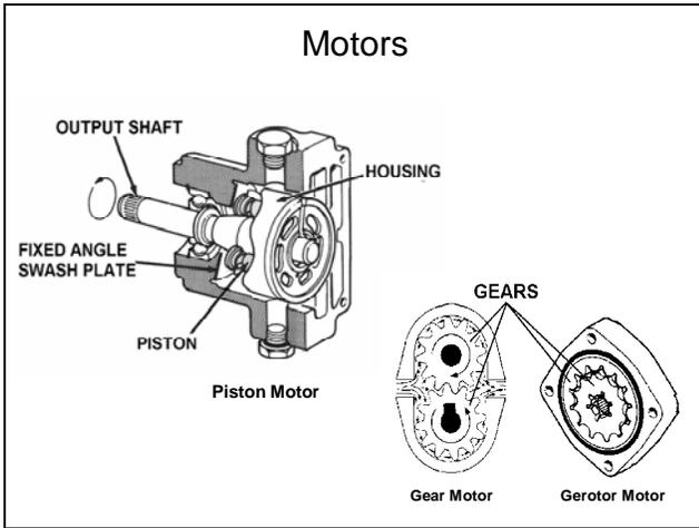
On a remote hydrostatic motor type system the hydrostatic motors can be a gear motor, gerotor motor or a piston type motor as shown here. On some designs a single motor is used to drive a differential transaxle. Another design uses individual motors for each wheel, either driving the wheels directly or through a planetary gear drive.
