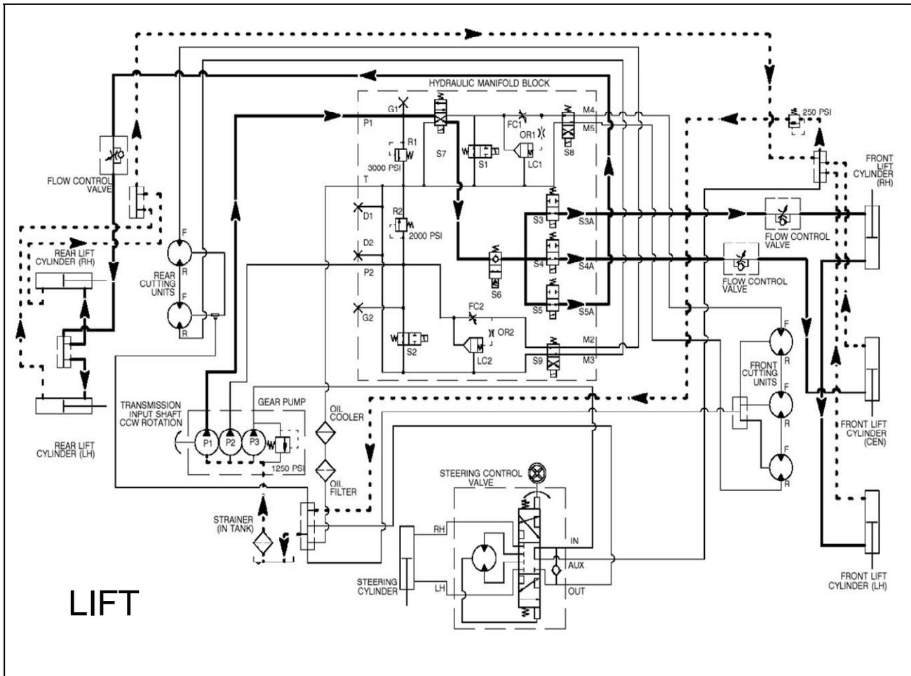
The key to understanding complex schematics is to break them down into their individual circuits. If you are troubleshooting a lift/lower problem, you don't need to be looking at the cutting drive or steering circuits.
