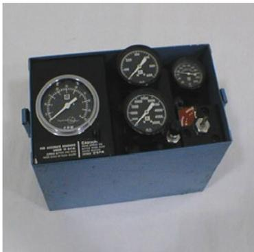
Higher capacity flow meters are also available from various sources. This particular one has 600 and 5000 PSI pressure gauges, a 10 GPM flow meter and a temperature gauge.
