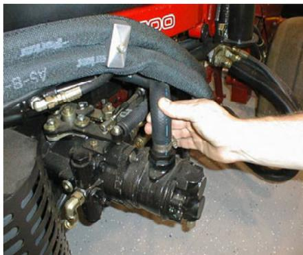
All hydraulic test should be made with the hydraulic system at normal operating temperature. Check for soft or collapsed suction hose.
