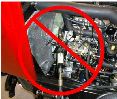
Position the tester hoses so that rotating machine parts will not make contact with them and result in hose damage.
