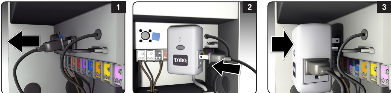
The EVO-AR works with any residential transformer with an internal AC outlet. One can also plug the AR unit directly into a wall outlet and then plug an electronic device into the AR's own outlet, such as holiday lights or a fountain.
