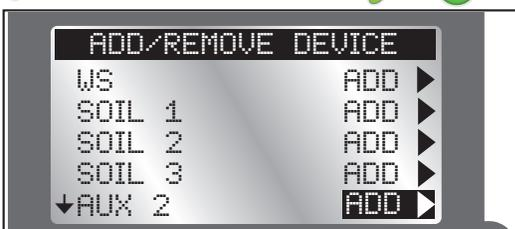
5. The EVOLUTION controller prompts the user to press the button on the AR to link the devices immediately.
