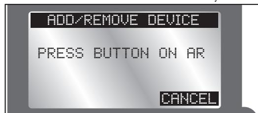
6. Press the Setup button on the Auxiliary Relay unit.
